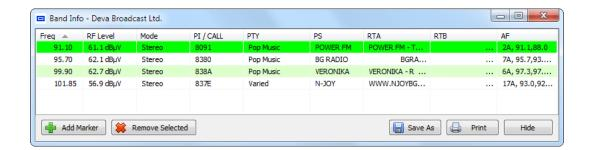
Band Info Table represents an additional information from the Analyze of the frequency band. Besides frequency, PI/CALL, PTY and PS, are shown station mode (stereo or mono), RF Level, Radio Text A&B and AF List if during the period of peak analyze there were enough RDS data to extract AFs.
