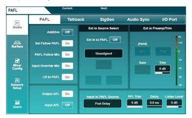
Touch any button on the left of the screen to turn an option on or off.
