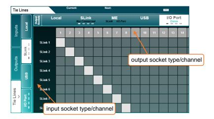
Tie lines are used to patch connections between source and destination points without using channel processing.
