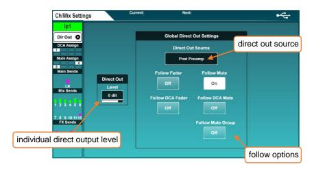
Touch the 'Dir Out' button on any input channel.
