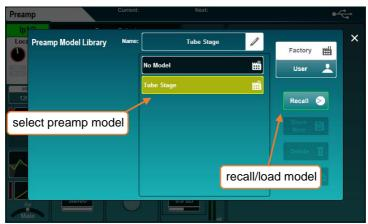
• Select a preamp, then press the 'Recall' button to load it.
