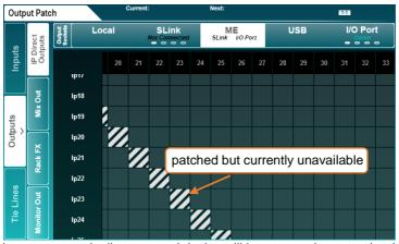
(i) All patching to a currently disconnected device will become active once the device is connected.
