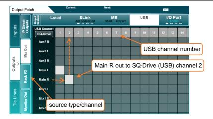
USB patching is for SQ-Drive or USB-B streaming connections. SQ-Drive uses input and output USB channels 1 to 16 and USB-B uses input and output USB channels 1 to 32.
