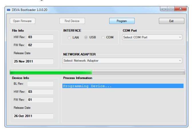
9. Firmware Upgrade completion is indicated by the progress indicator and in Process Information area as shown on the picture below:
