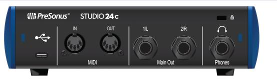
**Headphone Output.** The rear-panel headphone output mirrors the same streams as the Main left/right outputs.
