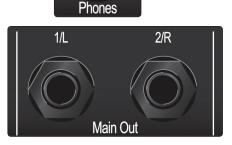
**Main Outs.** These are the Main outputs for the Studio 24c. The output level of the Main outputs is controlled by the Main level control on the front of the unit. Playback streams 1 and 2 are routed to these outputs.
