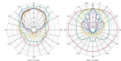
NOTES. 1.Frequency response: referred to 1 m; low end obtained through the use of near field techniques; one-third octave smoothed for correlation with human hearing, 5.Polars were acquired by placing the unit on a computer controlled turntable inside our anechoic chamber. Measurement distance was 4 m.
