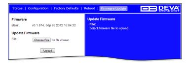
To update the device firmware, please select the new firmware file. Press the Upload button. A dialog window will appear. Confirm firmware update and wait for the process to complete.
