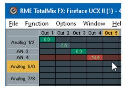
To maintain overview when the window size has been reduced, the labels are floating. They won't leave the visible area when scrolling. A right mouse click on the labels brings up the context menu with the exact same options as in the mixer view: Copy / Mirror / Paste /Clear input channels and submixes.
