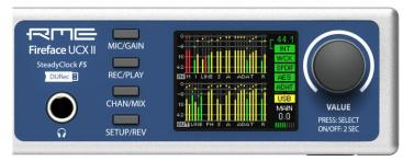
When the Global Level Meter screen is shown, the rotary encoder sets the monitoring volume of Main Out directly at the device. Pushing the button will change to Phones volume control, as indicated in the right lower corner of the screen.
