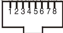
RJ-45 socket (front view):
