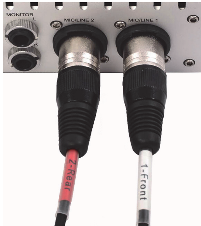
Figure 2-1 Connecting Sphere mic to the preamp
